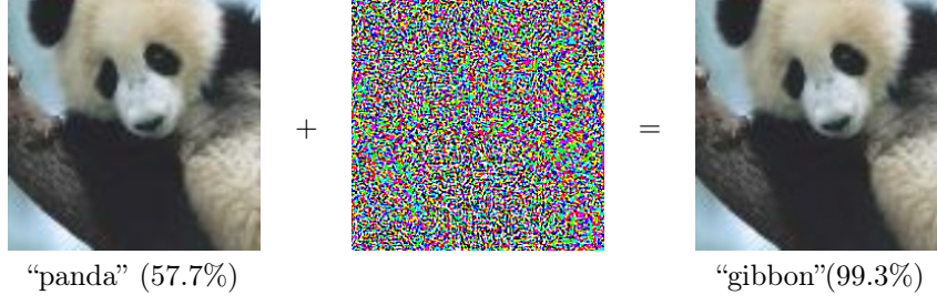
Figure B.1: A demonstration for adversarial example. Left: initial sample. Middle: adversarial noise. Right: adversarial example. We see that by adding an imperceptible noise, we can change significantly output compared to the one of initial sample. Source: [Goodfellow et al. 2014b].
