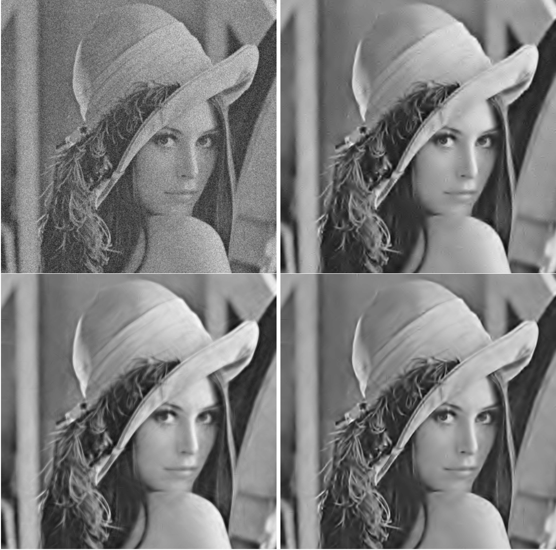
Figure 6. Noisy image (top left), and filtered images by the undecimated wavelet transform (top right), the curvelet transform (bottom left) and the combined transforms (bottom right).
